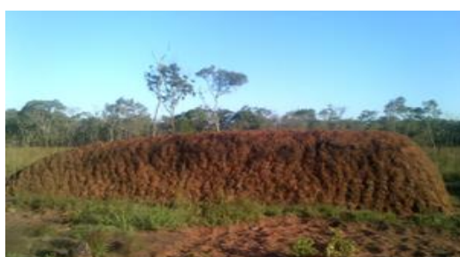
Figure 2: Traditional Charcoal Kiln
