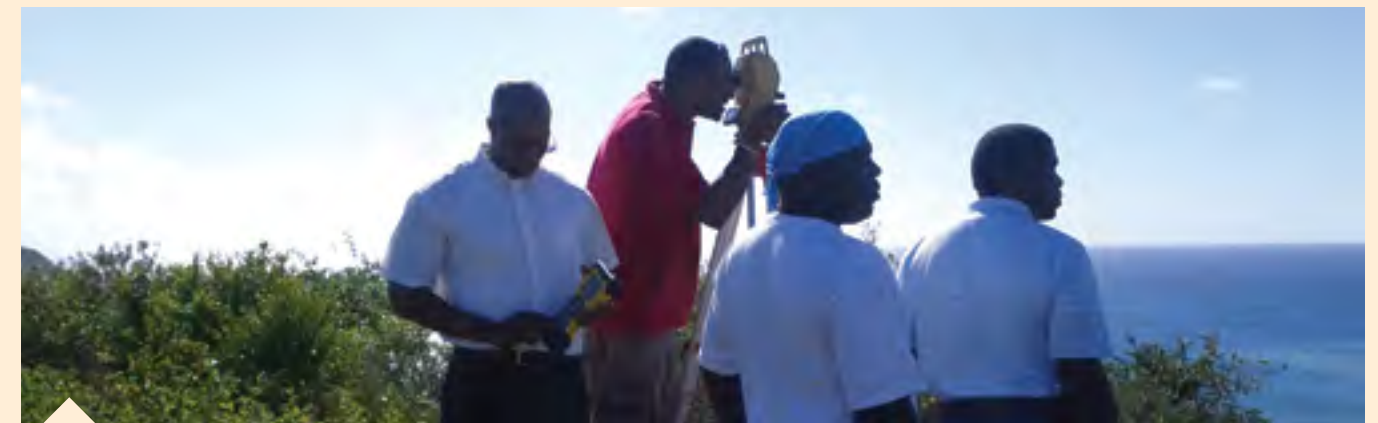
A team plots the coordinates of St. Lucia's West Coast highway with a portable GPS unit. The information will be loaded into St. Lucia's Integrated National Geonode (SLING), which was launched in March 2012 to inform better disaster preparedness and national planning. Photo: Jim Joseph
