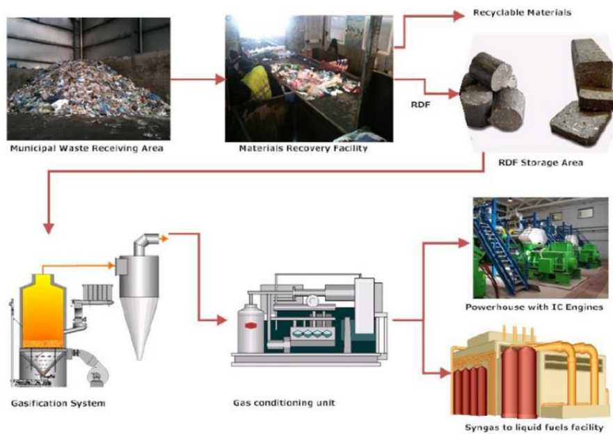
Figure 4.4: Production Cycle for Proposed Waste-to-Energy Facilities
